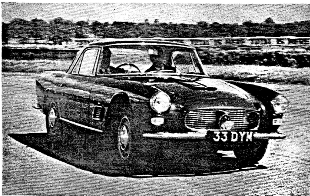
The Maserati 3500 G.T. which will go from 0 to 100 m.p.h. in fourteen seconds and has a maximum speed of over 140 miles an hour.
